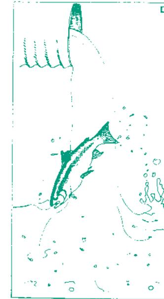
*Incorrect culvert installation can impede or prevent fish passage through a streamcrossing. Culvert conditions that block fish passage include: A) water velocities too great; B) water depths too shallow; C) insufficient resting area or jumping pool depth at culvert outlet; and D) culvert outlets that are too high above the streambed (Furniss, et al. in Handbook for Forest and Ranch Roads).*
