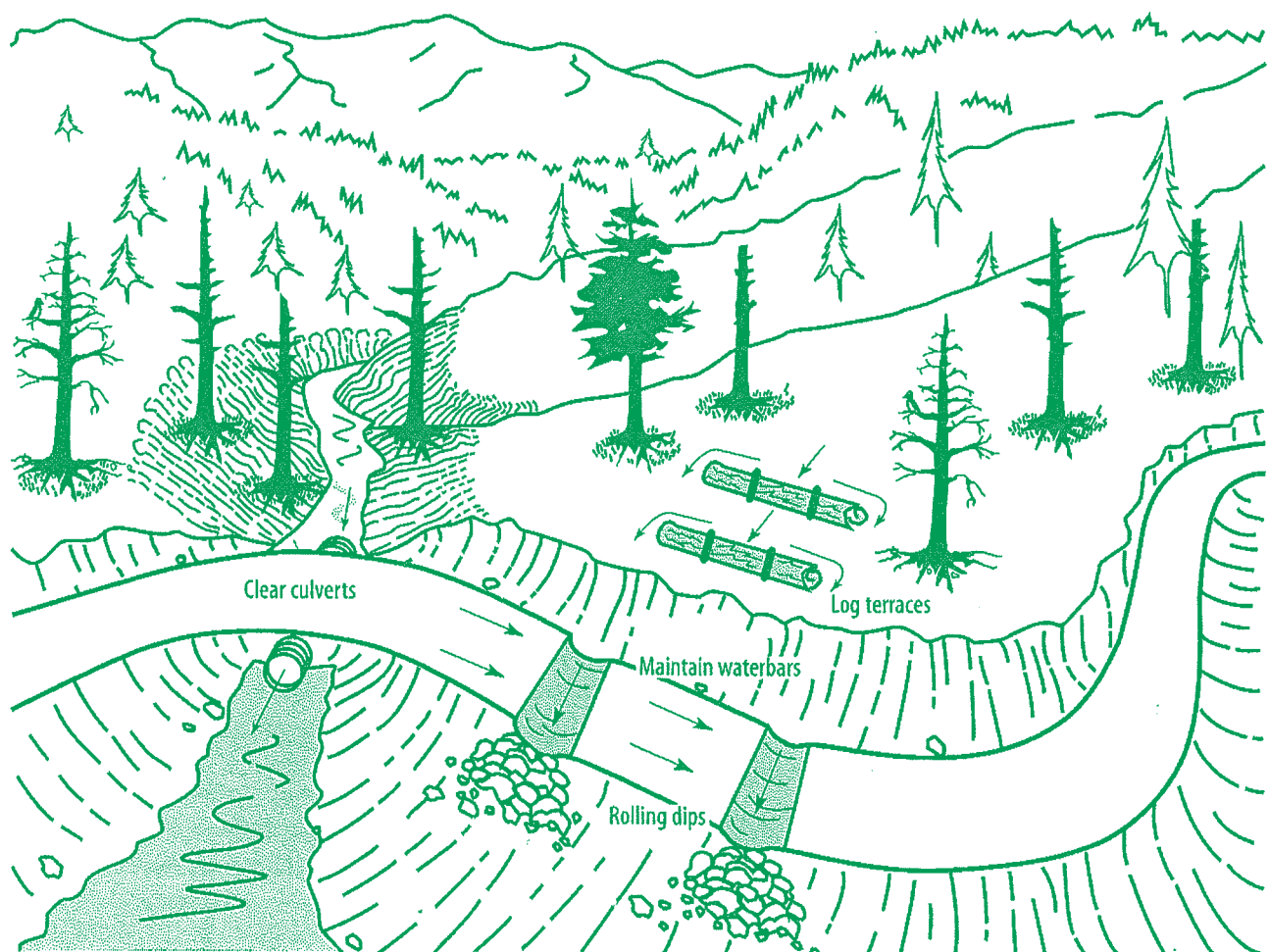
Erosion control and road maintenance practices (arrows indicate water flow). Adapted from Handbook for Forest and Ranch Roads (Mendocino County Resource Conservation District, June 1994) by Recovering From Wildfire, A Guide for California's Landowners.
